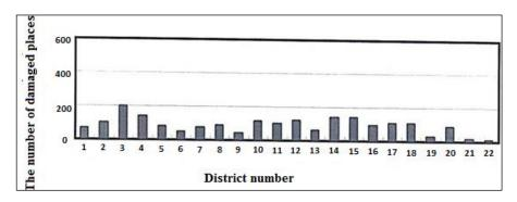
**Diagram 1.** The vulnerability of water supply pipelines in different districts of Tehran based on the floating model
