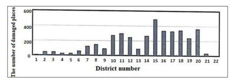
Diagram 2. The Vulnerability of water supply pipelines in different areas of Tehran based on Ray fault model
