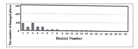
**Diagram 3.** The Vulnerability of water supply pipelines in different districts of Tehran based on the Fault model of the north of Tehran
