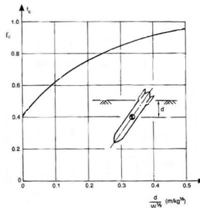
**Figure 2:** The coefficient of f<sub>c</sub> (force) based on the scale (Z)
