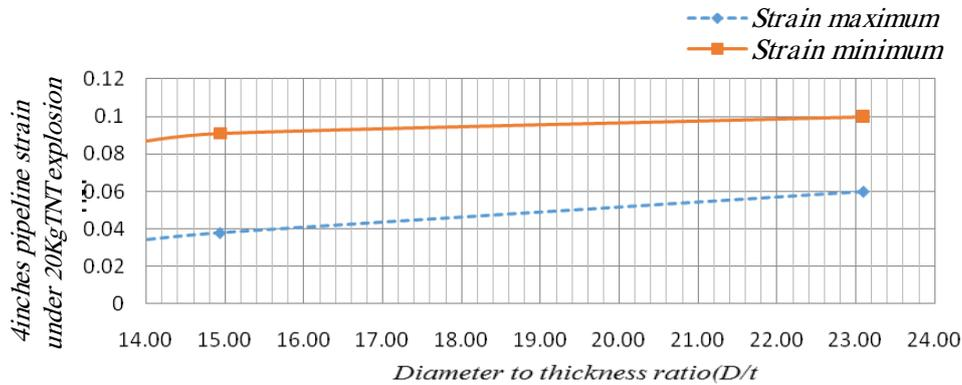
Figure 4: Effect of D/t ratio to the 4-inch pipe strain and explosion per explosive charge of 20 kg explosive material.
