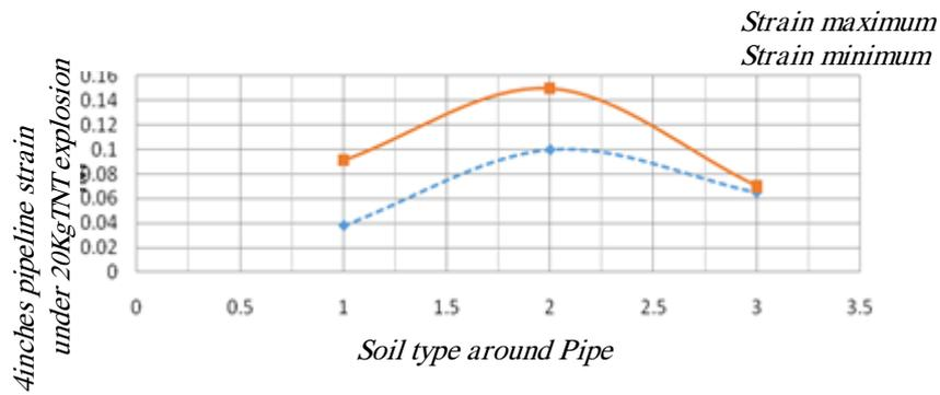
Figure 9: The effect of soil type on the behavior of a 4-inch pipe (1-sandy sand, 2-hardwood sand, 3- clayey soil)
