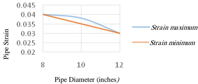
**Figure 6:** Impact of pipe diameter on pipe strain with depth of burial of 1 meter and explosion distance of 1 meter and TNT charge of 30 kg
