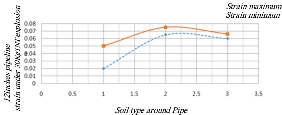
Figure 10: The effect of soil type on the behavior of a 12-inch pipe (1- soft sand, 2- hard soil sand, 3- clay soil)
