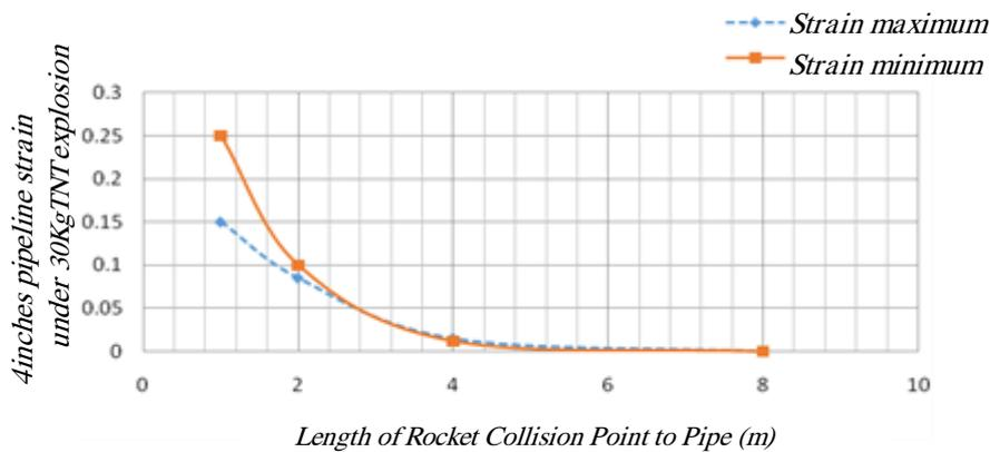
**Figure 8:** Effect of the Rocket Hit Site on the Strain of Pipe
