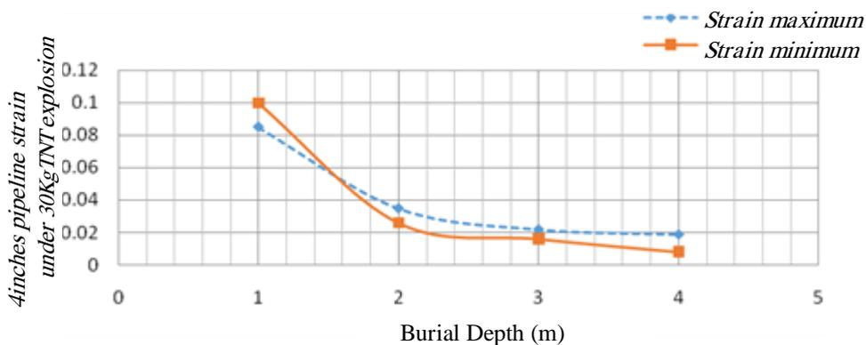
**Figure 7:** The effect of increasing the depth of pipe burial on the 4-inch pipe strain in explosion at 1-m distance
