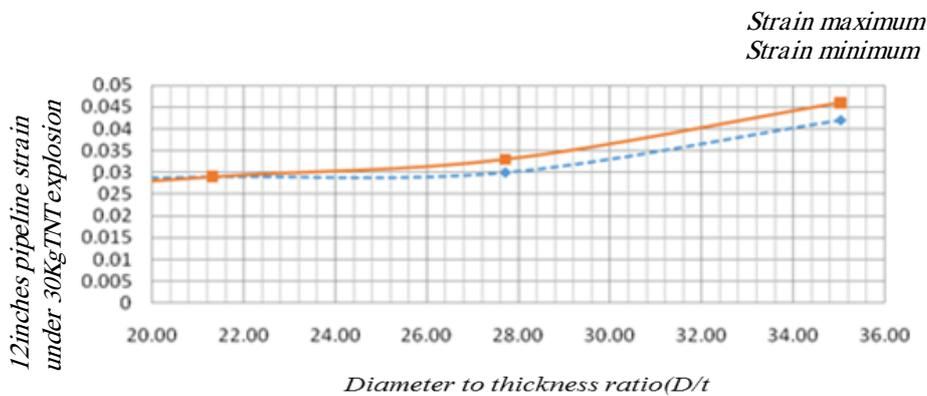
Figure 5: Effect of D/t ratio to 12-inch pipe strain due to explosive charge explosion 30 kg
